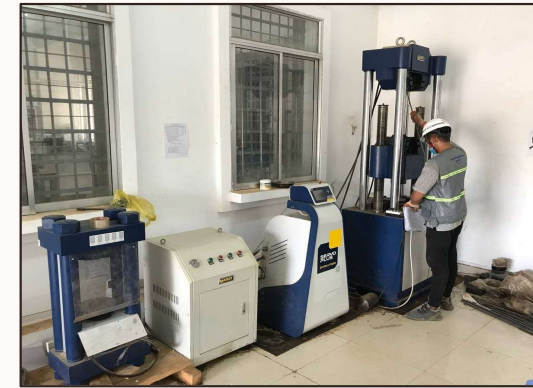
Tensile Strength Test of Steel
