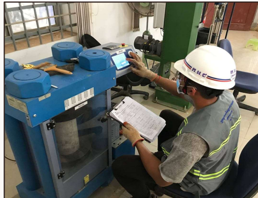
Compressive Strength Test of Concrete
